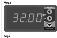
When lit, indicates that the reading is in Mega, (10<sup>6</sup>). 10,000K is shown as 10.00M and 1.0M as 1000K E.g.: 32.00 with M LED glowing indicates the value reads 32,000K
