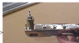
6) Mandrel removed from rivet tool
