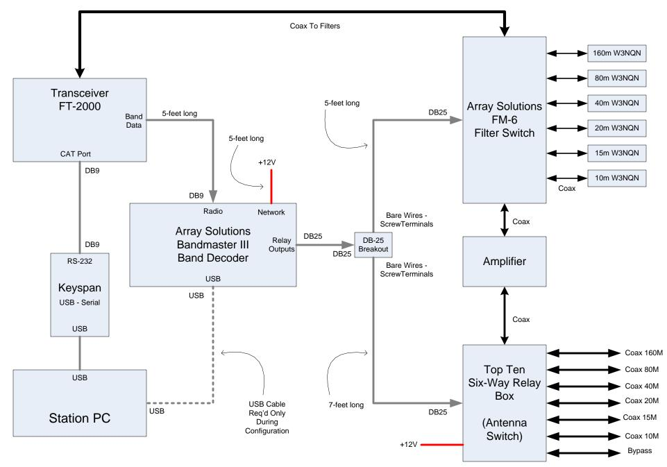
PJ2T Station 2 Filter & Antenna Switching
