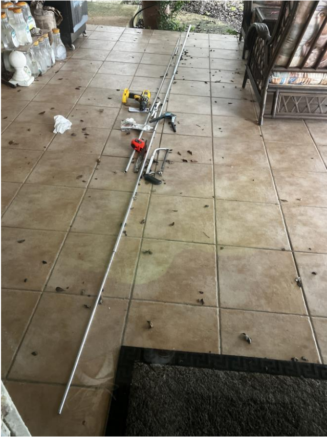
My workspace rebuilding the Ridge tribander 20 meter driven element during a massive downpour of rain.
