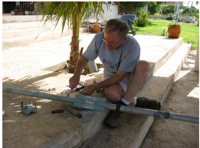
W0NB working on the boom of the 20 US/JA 5 element beam
