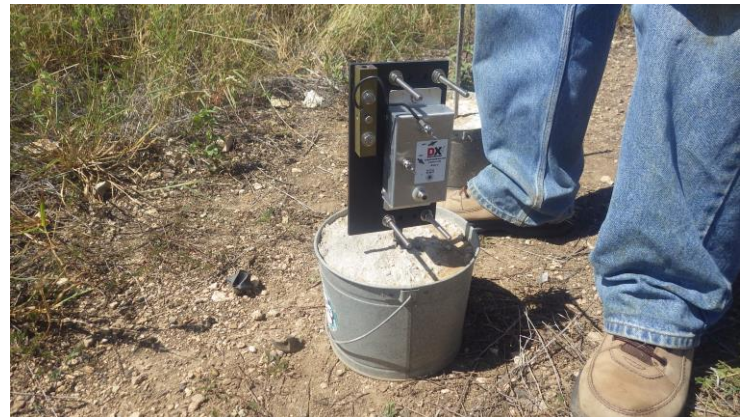
Jim and Jeff fabbed these portable concrete bases for the whips years ago.
