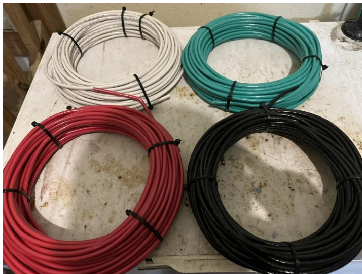
Four 100 ft lengths of #6 AWG to connect the gen to house (Photo W4IPC)
