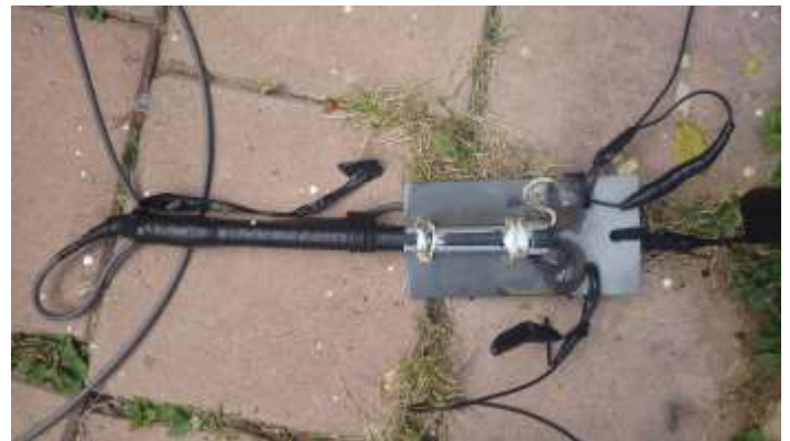
Feedpoint of the 80 2 el, with balun
