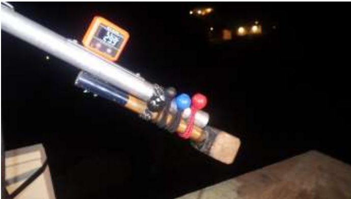
Expedient hand sledge hammer counterweight on the 1296 dish (photo W0CG). Note the elevation display.
