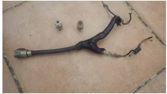
Bad pigtail and two bad barrels. The 20 foot piece of faulty RG-213 is not shown.
