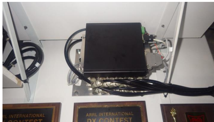
Closer view of the Bandmaster chassis and a bundle of 14 RG-8/X coax lines
