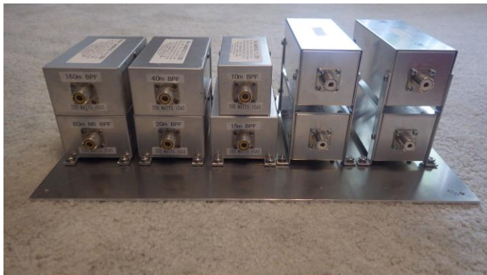
Filter block for the remote station
