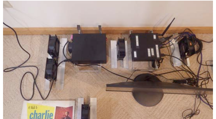
Airflow right to left, away from the wall at the right of the future shelf. The amp will be at the far left.
