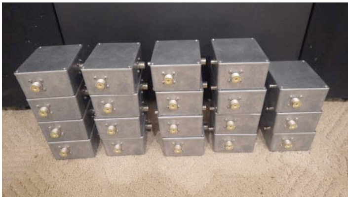
Completed coax relay boxes for the remote: 18 antennas and one spare box
