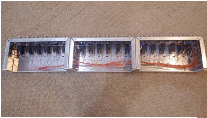
Another view of the 1 x 18 box, not quite complete. After the photo I shielded and bypassed the DC lines.
