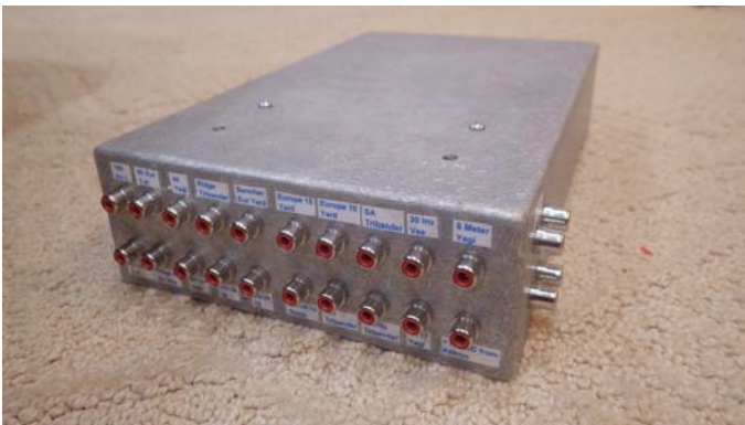
USB relay box with 23 keyed DC outlets and one input for +12 VDC from the Astron. The two USB ports are not visible in this view.
