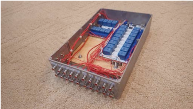
USB-controlled relay box, not quite complete. There are 24 contact closures available in this box, of which we are using 19. I laid in two spare boards to have on hand at Signal Point – these are inexpensive. After this photo I added 24 bypass caps at every DC input port.
