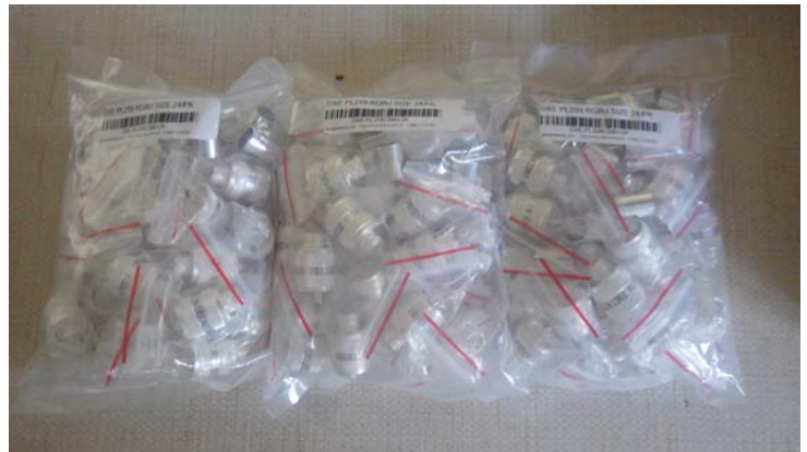
We will need a lot of coax jumpers to cable everything together. Here are the 72 crimp PL-259s donated by multiple members, acknowledged later.
