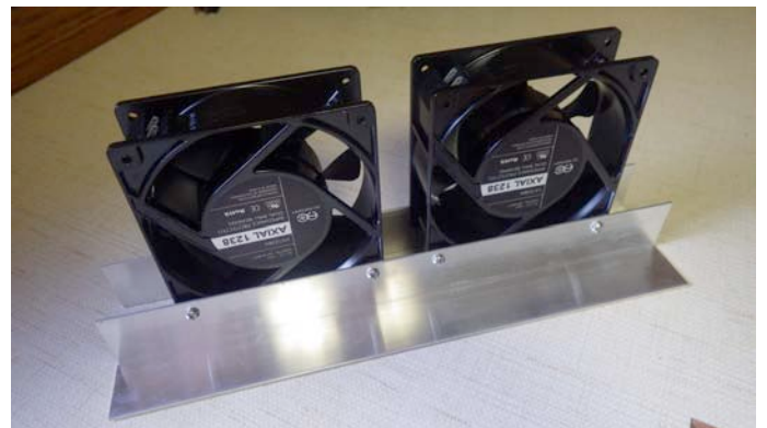
I made two of these double bank fan assemblies, one for the KPA amp and one for the K3. These are all lower RPM quiet fans, so they will not make a terrible amount of noise.
