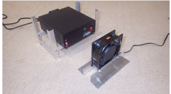
The homemade aluminum cooling rack for the Astron that elevates it so that air can flow freely around it.
