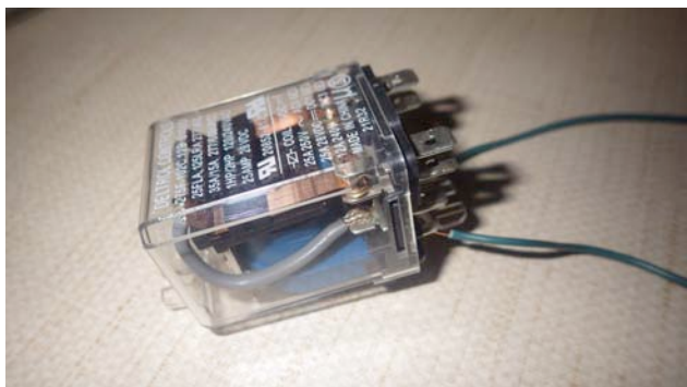
One of four Deltrol relays I bought to add to the W9NJY box to implement remote control.
