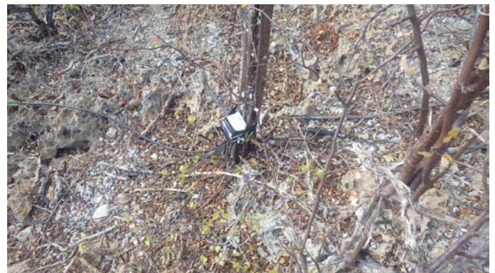
New feedpoint for modified Europe Beverage.
