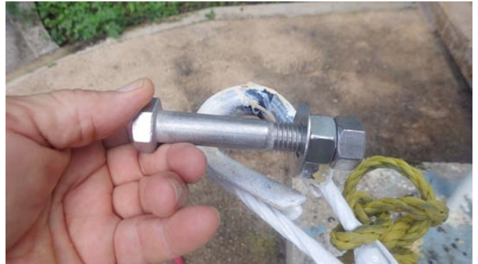
New stainless steel guy bracket bolt
