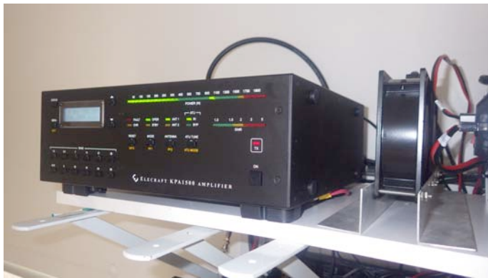
KPA-1500 with supplementary cooling blowing right to left in the photo
