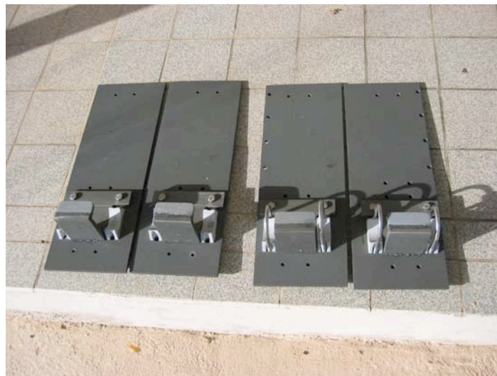
Corrosion-proof side yagi side mount brackets by N8LGP, September, 2006
