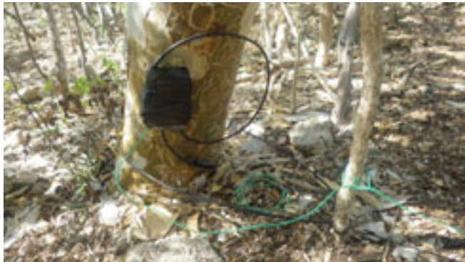
Feedpoint of the “upper” US/JA Beverage
