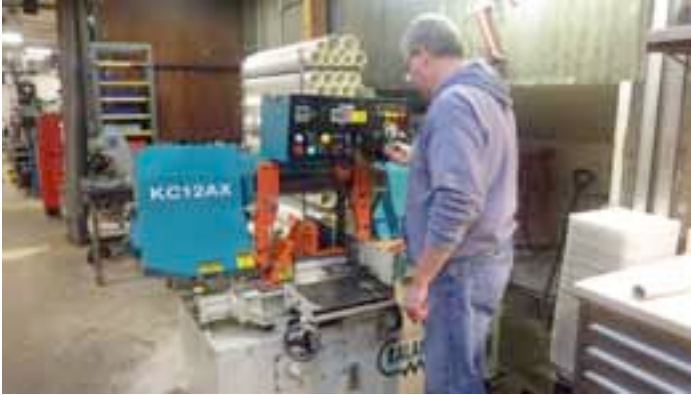
The photo shows Clarence Cook, owner of Kootenai Machine in Coeur d Alene, using a band saw to convert one of the pieces of the stainless pipe into two half shells on February 3. Here's the result below.
