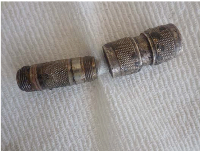
The failed Type N barrel on the left took out the entire Ridge system. It was burned black inside
