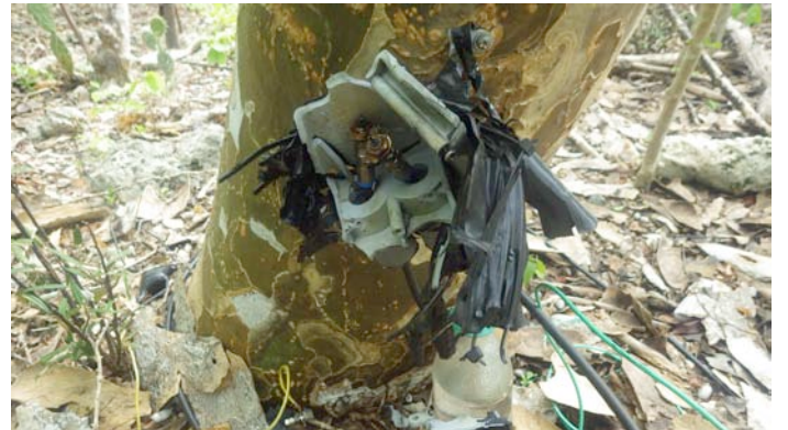
The lightning-blasted US/JA Beverage feedpoint
