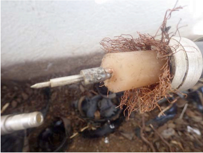
Center pin soldered correctly 13 years after installation
