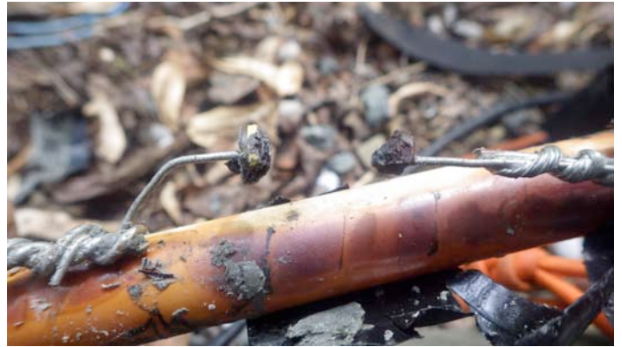
Europe Beverage termination blown to bits
