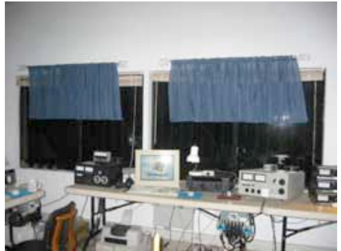
Station 2, circa 2003, with the Titan II amp (now dead), an FT-1000 Field (now dead), Windows 97 (now dead), a big CRT (now dead), an inkjet printer (now dead), manual antenna switches (now really dead), and YES! the LK-800 amplifier, still very much alive and serving us on 40 meters year after year.
