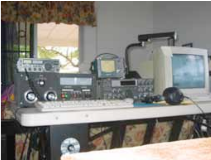
Above, a crude precursor to today's Station 4. A TS-930 (from W9VA), vintage Alpha 600 watt amplifier (from WI9WI), and a 45 pound CRT monitor.
