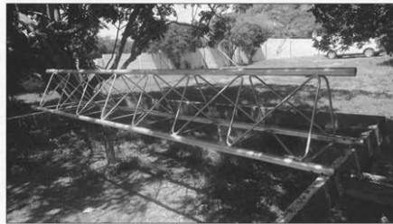
Figure 2 — This painting table at PJ2T makes section painting fairly easy.
