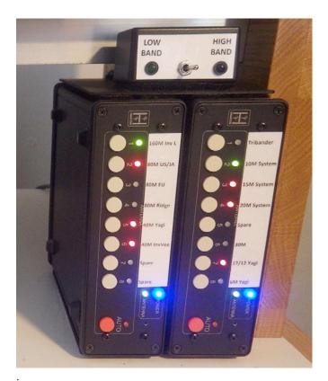
When you push this button you have immediate access to our four triband beams without having to use the 20, 15, or 10 meter system boxes (pictured below).
