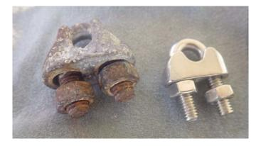
We installed up the clamp on the left on December 5 because I was short six stainless clamps. It was new, shiny zinc. This was for the overhead boom truss on the Bencher Europe Yard antenna. After nine weeks this is what it looked like, in contrast to the stainless steel clamp on the right. The original 2001 tower turned brown in very few weeks just the same as this clamp did.
