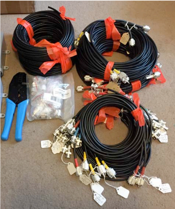
Figure 9: Cables to rewire receive antenna switching system.
