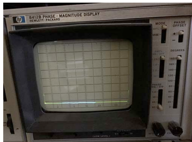
Figure 6: Transmission loss of 50 ohm fed line choke
