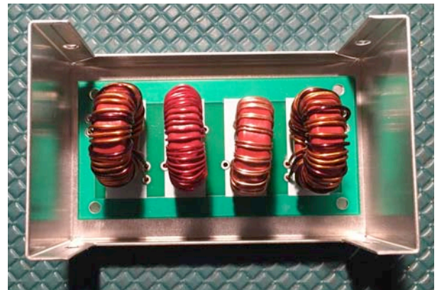
Figure 3: 160 meter W3NQN receive band pass filter board in its utility box.
