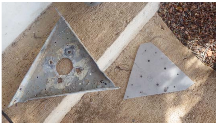
Old rotor plate and the W0CG custom stiffener before they were bolted together.
