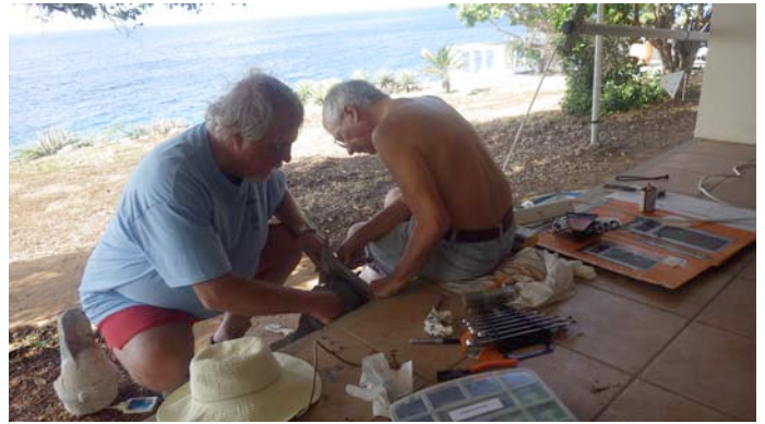
VE3CX and W0CG mating the stiffener to the old rotor plate with six sets of stainless screws, washers, and fiber nuts.
