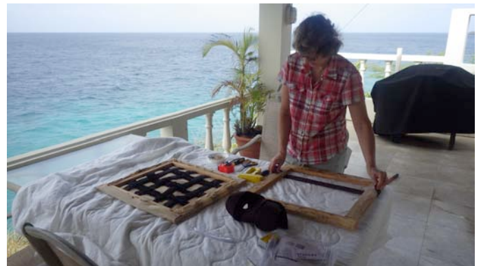
Wrestling out hundreds of old staples to remove the failed seat webbing.
