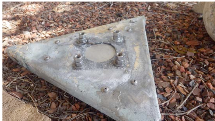
Rebuilt WARC rotor plate, ready for installation.
