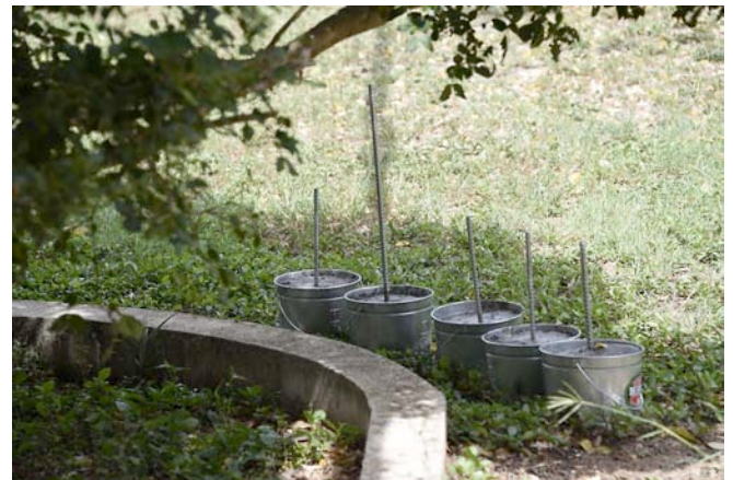
Portable concrete buckets bases for the 4SQ by W8WTS and K8ND
