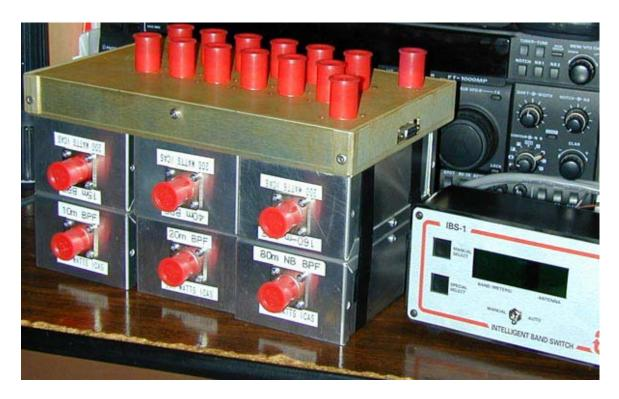
The above picture shows the FM-6 on top of 6 W3NQN Filters, which are strapped together. The coaxial cables will be routed next around from the FM-6 to each individual filters input and output connector.
