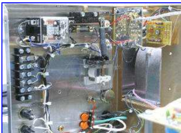
Factory Installed New Relay Board (courtesy of K5JP)
