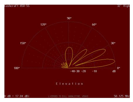
Figure 7: Modified A50-5S Elevation Plot
