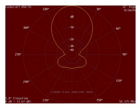
Figure 4: Stock A50-5S Azimuth Plot
