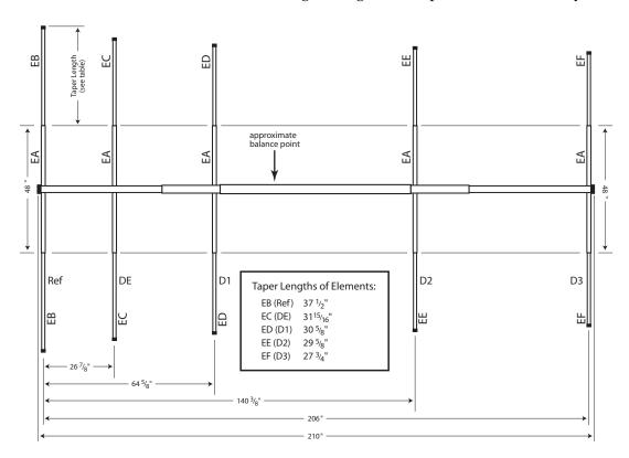
Figure 2: Reassembled Antenna Dimensions
