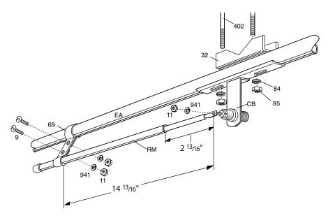
Figure 3: Gamma Match Configuration Showing Adjustment Dimensions
