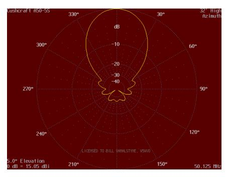
Figure 5: Modified A50-5S Azimuth Plot
