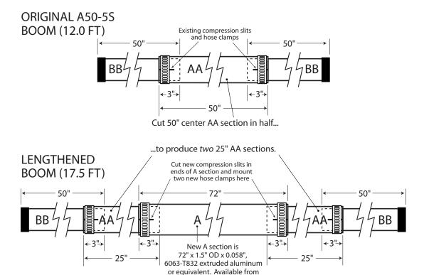
Figure 1: Original and Lengthened Boom Assembly
