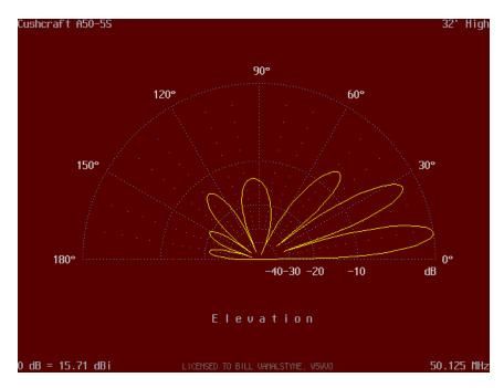
Figure 6: Stock A50-5S Elevation Plot
